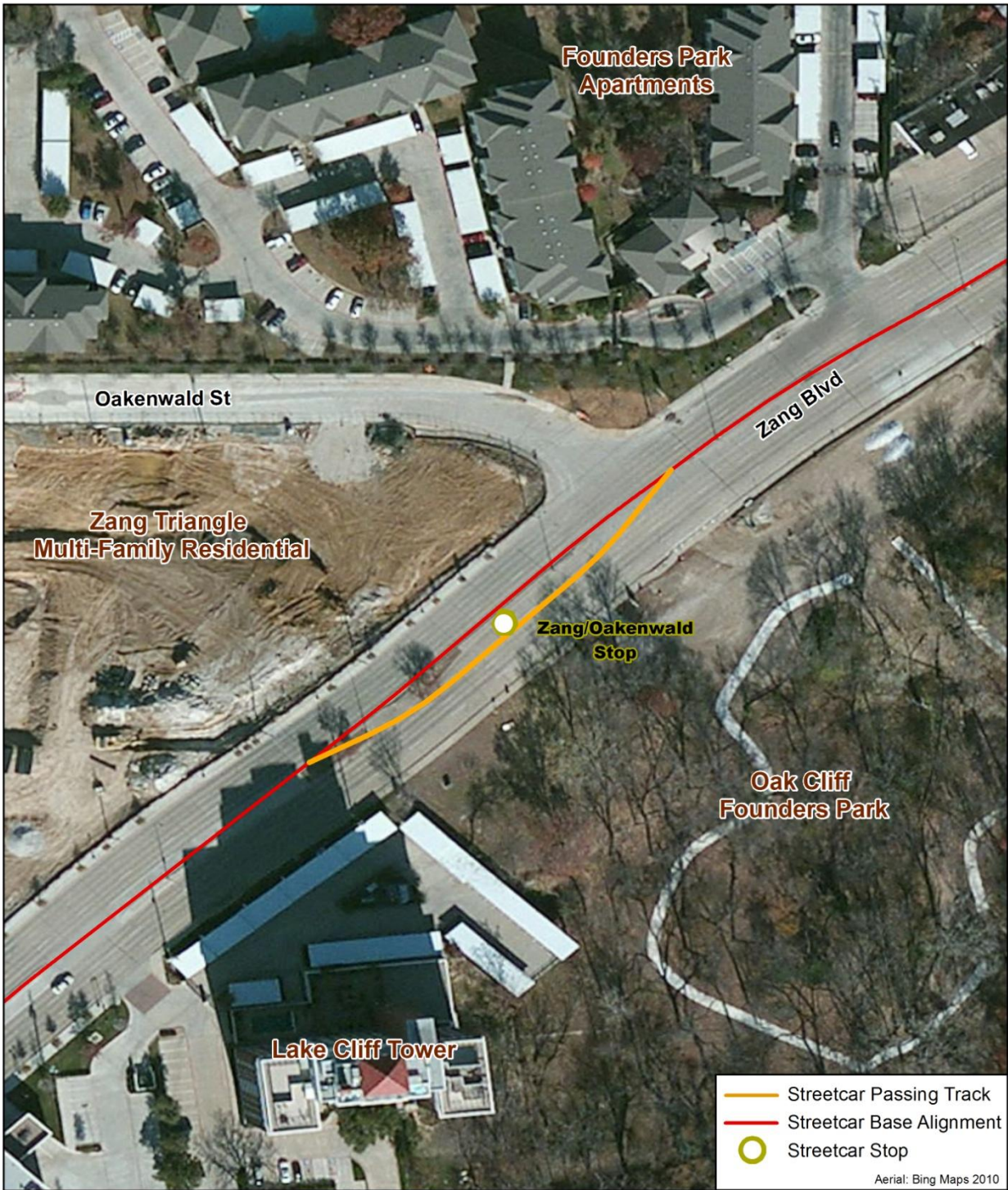
Figure 2 Union Station to Oak Cliff Streetcar TIGER Passing Track Project Location 0 50 100 Feet N DART | gpc 5
