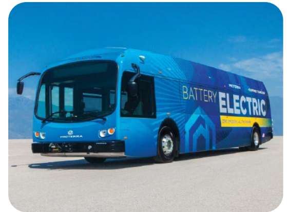
Proterra "ZX5" -- 40' Long-Range Battery Electric Bus
