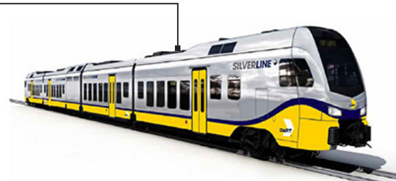
The DART Silver Line will have eight diesel-electric vehicles built by Stadler Inc.
