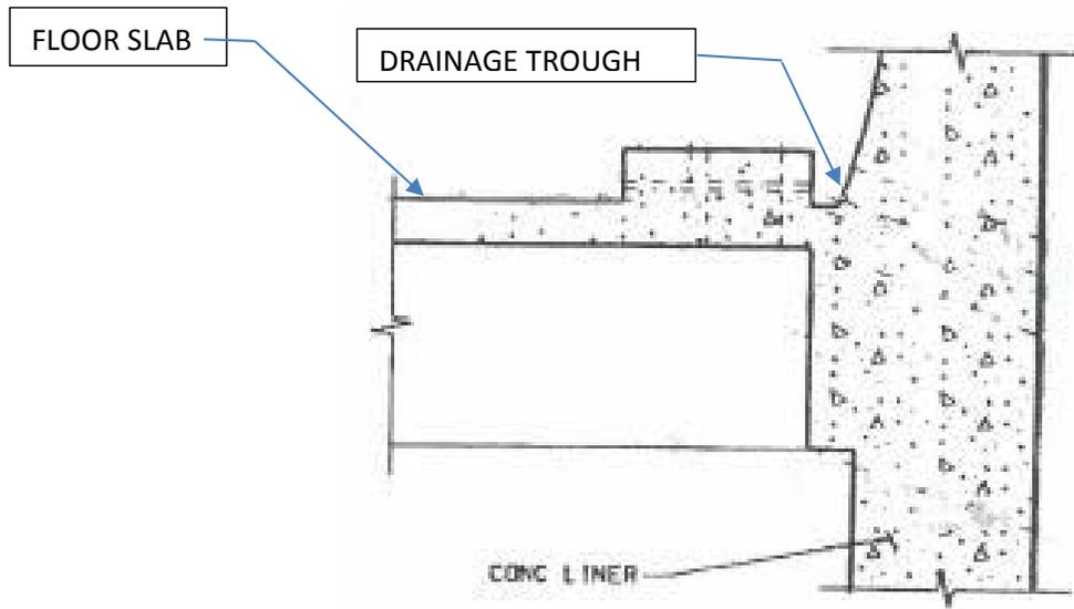
**FIGURE 2: TYPICAL DETAIL of DRAINAGE TROUGH for INTERNAL WATER DRAINAGE**
